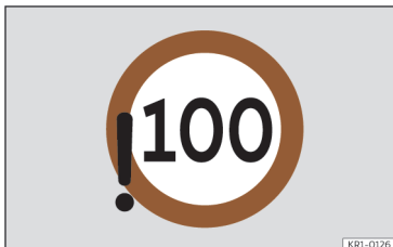
Fig. 10 On the instrument cluster screen: violation of the detected speed limit (illustration).
