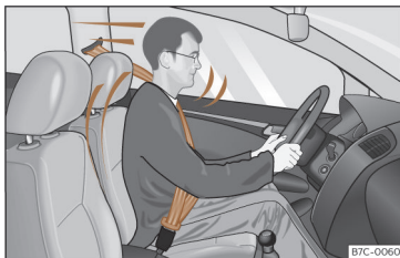
Fig. 19 Drivers with properly worn seat belts will not be thrown forward in the event of sudden braking.
