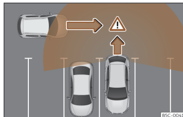
Fig. 164 Diagram of the parking assistant: detected area around the vehicle that is driving off.
