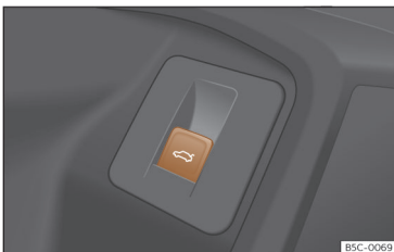
Fig. 83 On the driver's door: button for opening and closing the rear lid.
