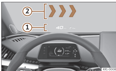
Fig. 4 In the driver's field of view: Proximity HUD ① and AR HUD ②.
