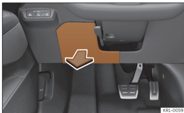
Fig. 191 On the dashboard on the driver side: lid of the fuse box.
