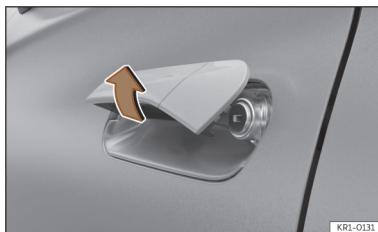
Fig. 72 Mechanical door opening.
