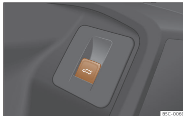
Fig. 78 On the driver's door: button to open and close the rear lid.
