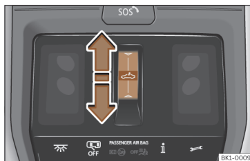
Fig. 101 On the interior roof lining: function button to operate the sun blind.
