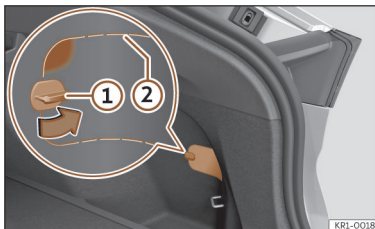
Fig. 61 On the lower right-hand side of the luggage compartment trim: cover with cutting lines.
