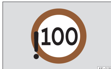
Fig. 8 On the instrument cluster display: violation of the detected speed limit (illustration).
