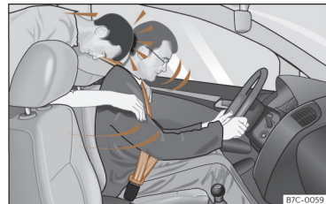
Fig. 19 Any rear seat occupants not wearing a seat belt may be thrown forward violently, hitting the driver who is wearing the seat belt.
