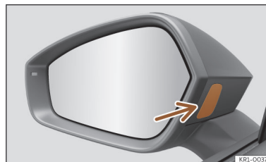
Fig. 153 On the mirror: warning lamp.
