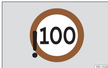
Fig. 9 On the instrument cluster display: violation of the detected speed limit (illustration).
