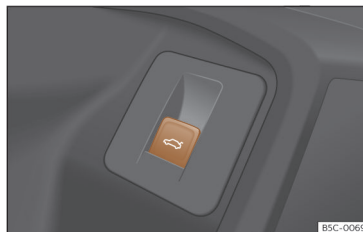
Fig. 85 On the driver's door: button to open and close the rear lid.
