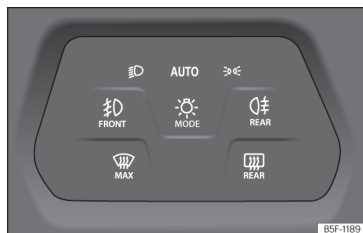
Fig. 107 Instrument panel: light panel.
