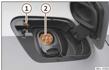
Fig. 56 Behind the battery charging cover on the rear right-hand side: Charging socket
