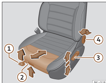
Fig. 84 Front seats: manual seat adjustment.
