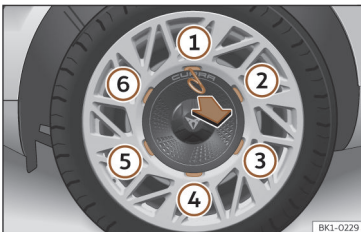
Fig. 192 Changing the wheel: removing the central trim.
