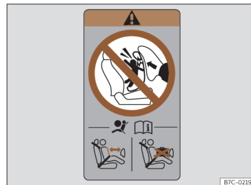
Fig. 35 Airbag sticker: on the rear frame of the passenger side door.
