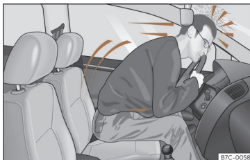
Fig. 18 A driver not wearing a seat belt may be thrown forward violently.
