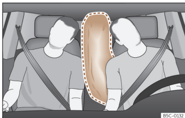
Fig. 29 Fully inflated central airbag (deployment zone).
