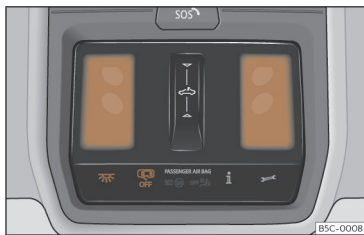
Fig. 95 Detail of headliner: front interior lighting.
