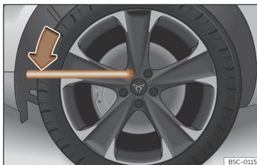
Fig. 195 Tyre change: loosen the wheel nuts.
