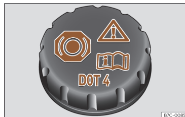
Fig. 187 Front compartment: brake fluid reservoir cap.
