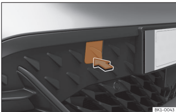
Fig. 177 Front bumper on right: remove the lid.
