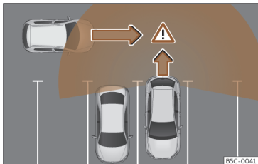
Fig. 147 Diagram of the parking assistant: detected area around the vehicle that is driving off.
