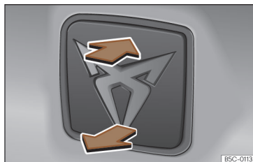
Fig. 78 Rear lid: opening from the outside.
