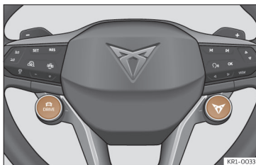
Fig. 108 Multifunction steering wheel: DRIVE and CUPRA buttons for selecting and changing the drive profile.
