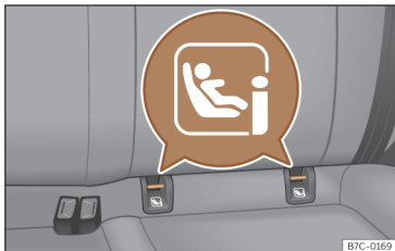
Fig. 36 Rear seat: location of the ISOFIX or i-Size securing rings.
