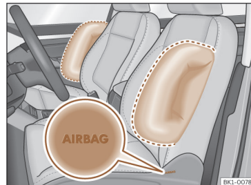
Fig. 30 Driver's seat and passenger seat side airbags.
