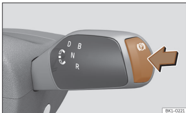
Fig. 133 On the gear selector: electronic parking brake button.
