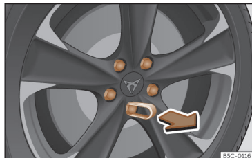
Fig. 193 Wheel: wheel nuts with caps.
