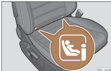
Fig. 37 Front passenger seat: location of the i-Size securing rings.
