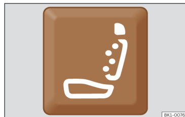
Fig. 92 On the lower side of the driver and passenger seats: massage function button.
