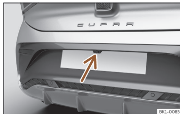
Fig. 114 On the rear bumper: location of the rear assist camera.
