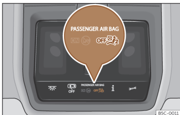
Fig. 27 On the roof console: passenger airbag deactivation control lamp.
