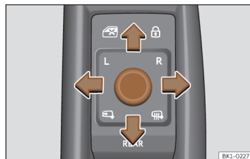
Fig. 99 Driver's door detail: exterior mirror control.
