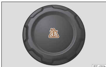
Fig. 186 Front compartment: coolant expansion tank cap.
