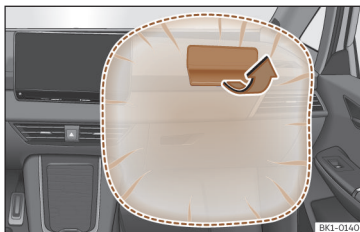
Fig. 25 Front passenger airbag located in dash panel.
