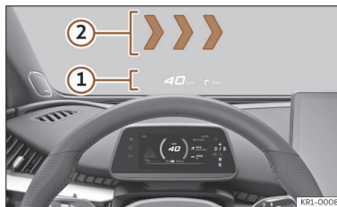
Fig. 5 In the driver's field of view: Proximity HUD ① and AR HUD ②.
