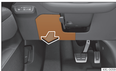
Fig. 190 On the dashboard on the driver side: lid of the fuse box.
