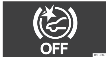
Fig. 127 On the screen of the instrument panel Front Assist switched off message.
