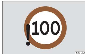
Fig. 9 On the instrument cluster screen: violation of the detected speed limit (illustration).
