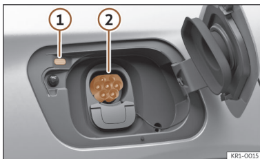
Fig. 56 Behind the battery charging cover on the rear right-hand side: Charging socket
