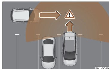
Fig. 151 Diagram of the parking assistant: detected area around the vehicle that is driving off.
