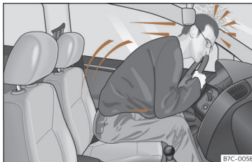
Fig. 19 A driver not wearing a seat belt may be thrown forward violently.
