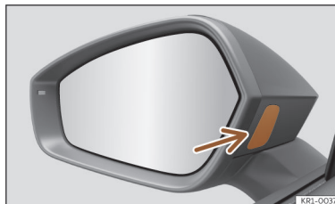
Fig. 153 On the mirror: warning lamp.
