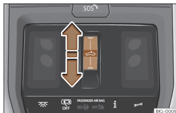
Fig. 100 On the interior roof lining: function button to operate the sun blind.
