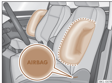
Fig. 31 Driver's seat and passenger seat side airbags.
