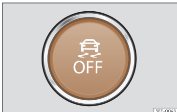
Fig. 126 On the lower part of the centre console: ESC on/off button
