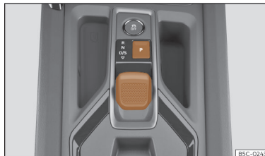
Fig. 123 On the centre console: selector lever.
