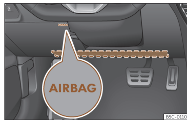
Fig. 34 On the driver side: location of airbag for knees.
