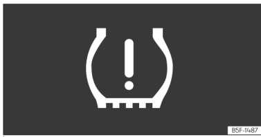
Fig. 240 Instrument cluster: warning of loss of tyre pressure.
