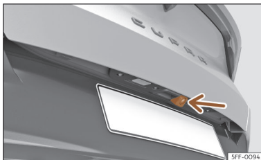
Fig. 133 On the rear lid handle: location of the rear assist camera.
