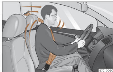
Fig. 17 Drivers with properly worn seat belts will not be thrown forward in the event of sudden braking.
