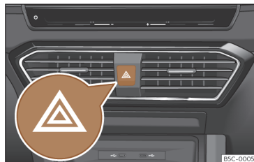
Fig. 49 Dashboard: switch for hazard warning lights.
