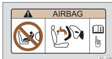
Fig. 37 Airbag sticker: on the passenger side sunshade blind.
