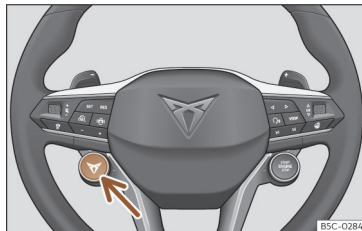
Fig. 125 Multifunction steering wheel: button to change the driving profile.
