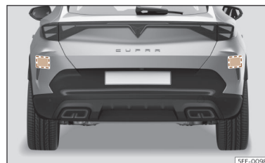
Fig. 131 Rear view of the vehicle: radar sensor areas.
