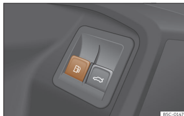
Fig. 201 Driver's door: tank cover release.
