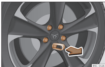
Fig. 235 Wheel: wheel bolts with caps.
