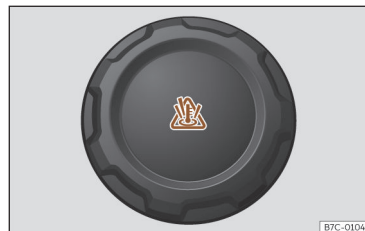
Fig. 219 Front compartment: coolant expansion tank cap.
