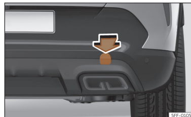
Fig. 210 Rear bumper on right: remove the lid.
