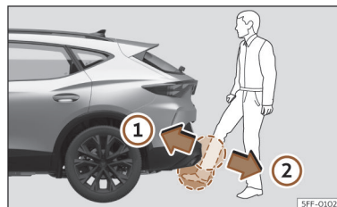
Fig. 84 Rear lid with sensor-controlled opening (Easy Open).
