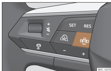
Fig. 127 Left side of the multifunction steering wheel: button for driver assistance systems (depending on the version).
