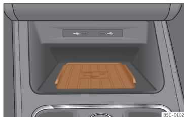
Fig. 181 On the centre console: pad for the mobile phone connection.
