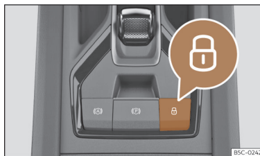
Fig. 77 On the centre console: central locking button
