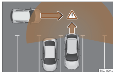
Fig. 166 Diagram of the parking assistant: detected area around the vehicle that is driving off.
